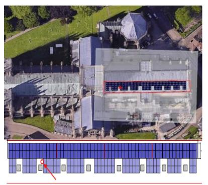
The Starlink dish will be securely mounted to the existing photovoltaic (PV) installation rail. No additional fixings to the cathedral structure will be required. The dish will be positioned discreetly behind the S9 pillar.
